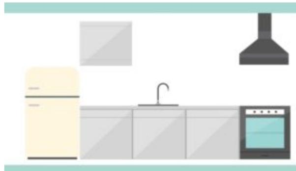
Kitchen service voids are empty spaces that are hidden from view once the units are installed. However, they're important for providing space for pipes and electrical supplies, and they are also used to ensure the units line up properly in corners. Prept kitchen cabinets all have a service void built in to make your planning and install as simple as possible.
